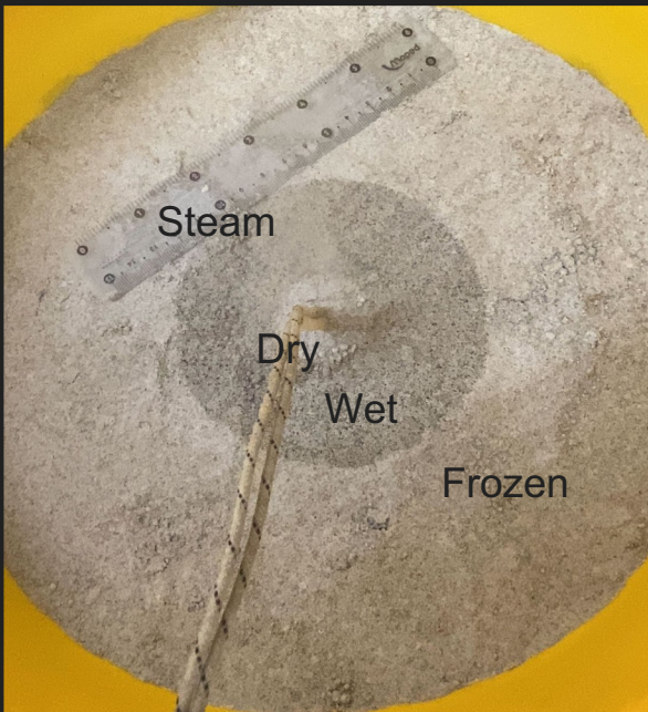
10wt% Frozen Water & MTU-LHT-1A @ Constant 100 Watts
