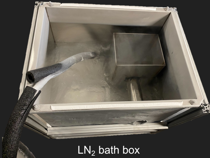
Insulated LN 2 bath box in fume hood
