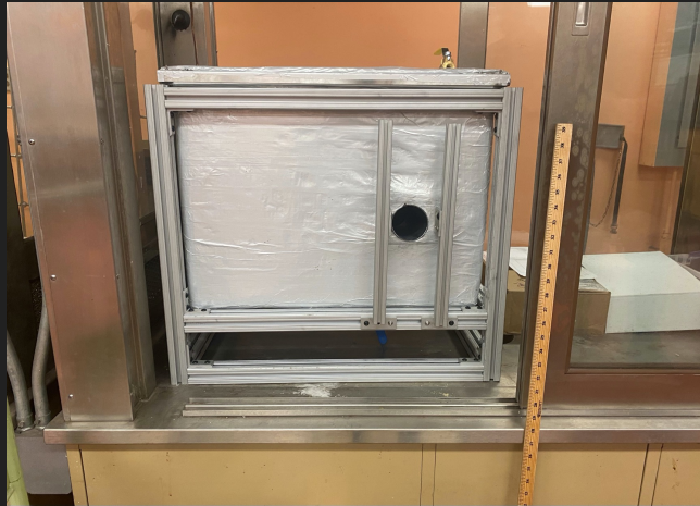
Insulated LN 2 bath box in fume hood
