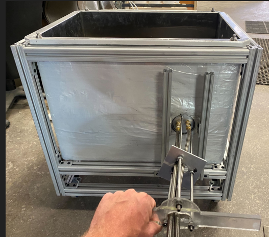
Volatile plunger and LN 2 box
